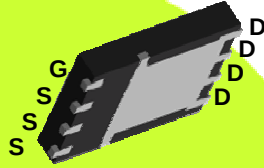
QFN 5mm x 6mm Plastic Package
