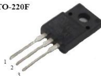
1. Gate 2. Drain 3. Source
