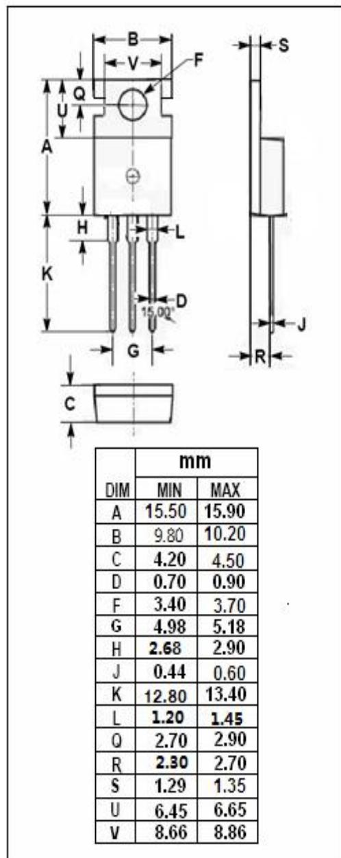
**isc Silicon NPN Power Transistor**
