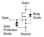
**Remark** The diode connected between the gate and source of the transistor serves as a protector against ESD. When this device actually used, an additional protection circuit is externally required if a voltage exceeding the rated voltage may be applied to this device.
